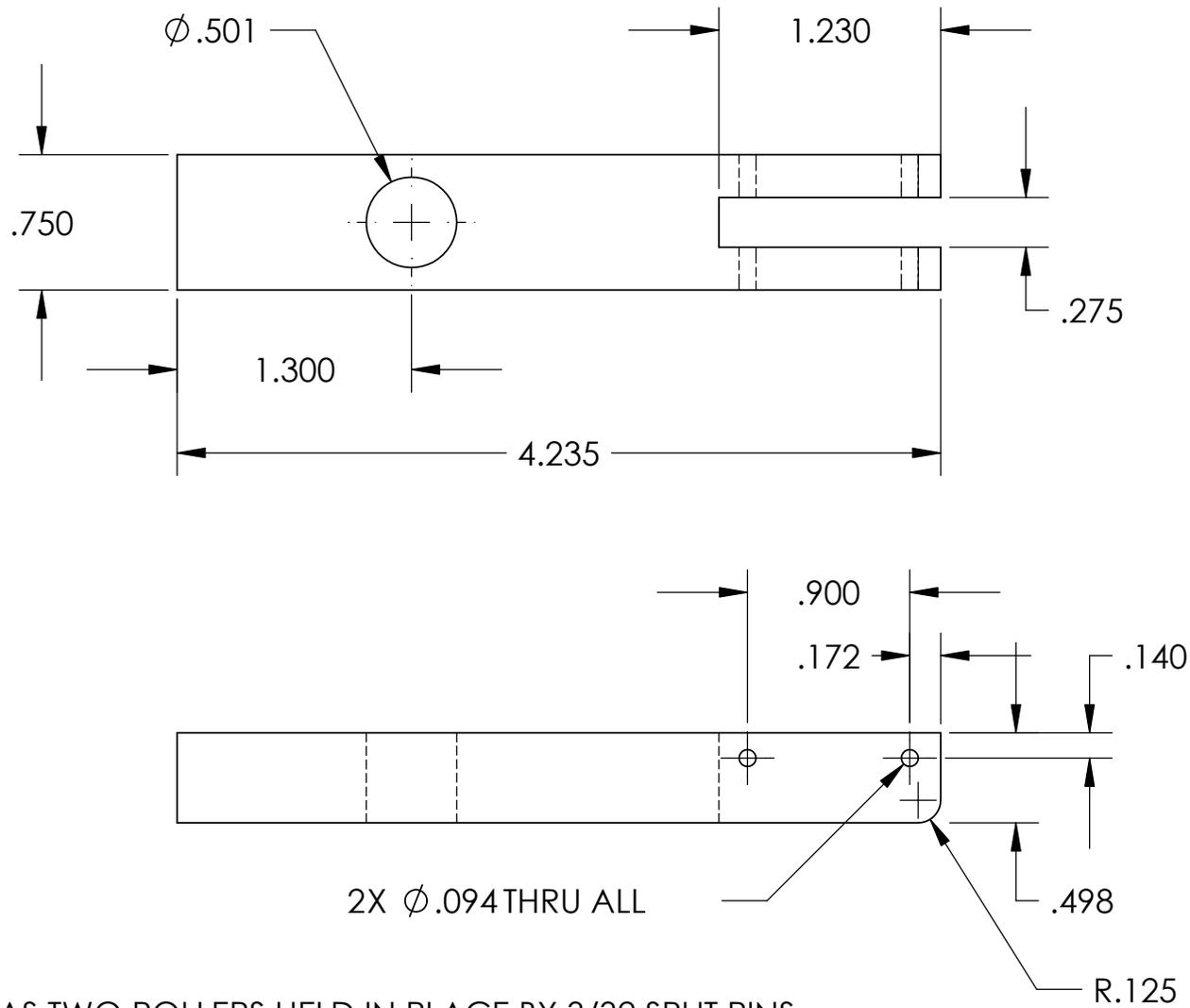
THE BAR HAS TWO ROLLERS HELD IN PLACE BY 3/32 SPLIT PINS.
