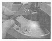
Clear the press of powder, primers, and good brass. Remove the Star safety cam assembly if present.
