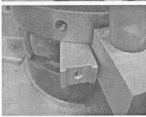
With fingers out of the way bring the press down and tighten the aluminum clamp on the rod up against the die plate and with the cutout parallel to the case feeder. This clamp will always be up against the die plate, but may need some fine adjustment left or right.
