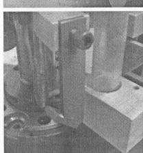
Cycle the press slowly to test for proper operation. On the down stroke, the fork finger should ride out, then snap over the angle cam. On the up stroke, the fork finger rides the other side of the cam and pivots the fork ejecting the case. If anything binds, you may have to rotate the aluminum clamp a little bit.
